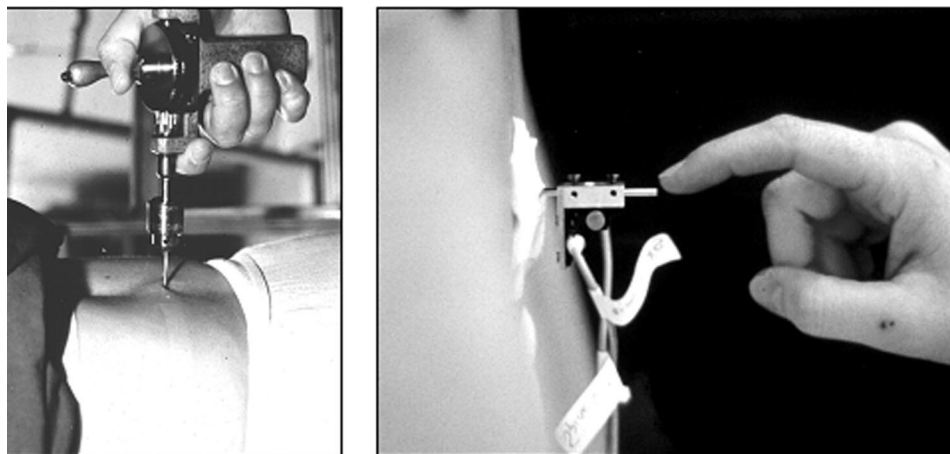
Figure 1. Pin placement in L4 (left) and the greater trochanter was performed under local anesthetic with the goal of placing the pins such that they were orthogonal to the bone under study. Accelerometers were then attached (right), and the pin "plucked" to determine resonance of the pin-bone system (L4 shown).
